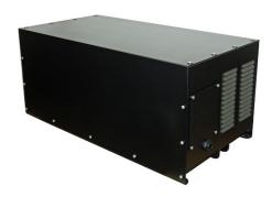
A MultiPhase efficiently converts single-phase into three-phase power much like a Booster converter. Its digital power electronics not only balances three-phase voltages during motor start-ups but also across all loads between 0% and 100%.
